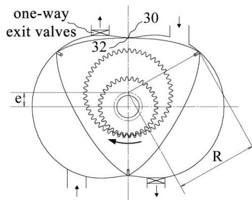
**Figure 1** A cross sectional view through the machine with rotor at ‘engine’ TDC (top dead centre) position.
