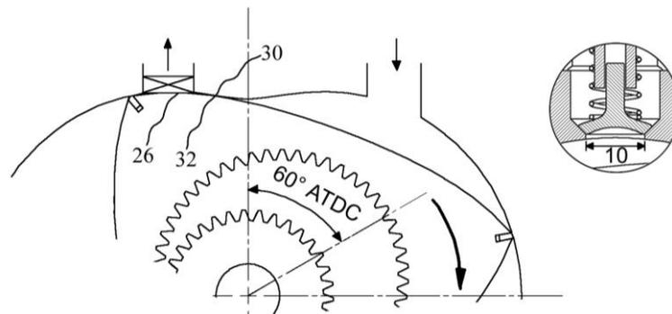
**Figure 2.** Nesting of the rotor flank with the housing bore at the end of the exhaust stroke; with an inserted view of an exit valve (three are fitted transversely)
