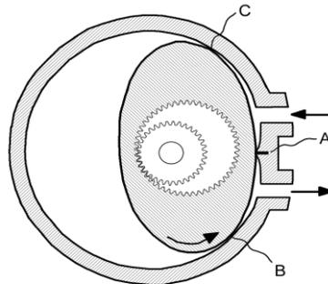
**Figure 4** Axial view of a *hypotrochoidal* type rotary piston vacuum pump
