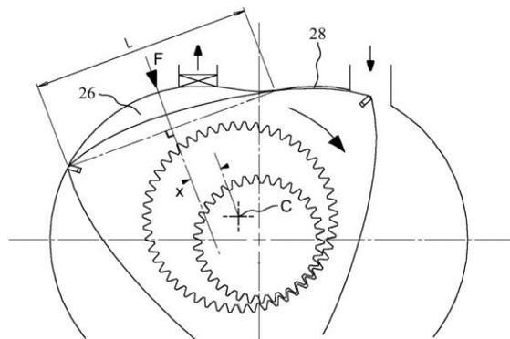
**Figure 3.** Intermittent torque loading on the gears results from the uneven gas pressure on the rotor flank. Pressure in chamber 26 is higher than in 28 resulting in Force F producing a torque  $Fx$  about the centre C of the rotor
